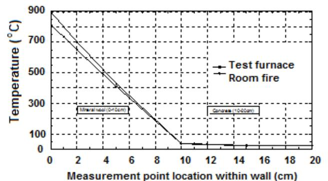
Figure 7 Temperatures achieved in construction after 3600s exposure – combined
