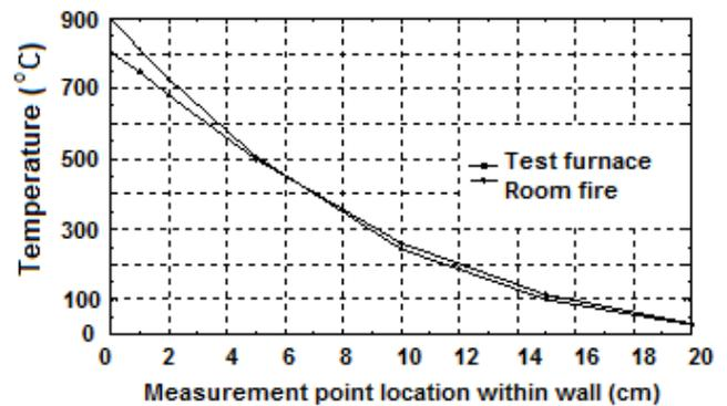
Figure 6 Temperatures achieved in construction after 3600s exposure – mineral wool
