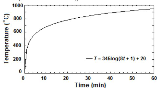
Figure 1 Standard time-temperature curve
