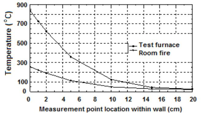
Figure 5 Temperatures achieved in construction after 3600s exposure – concrete
