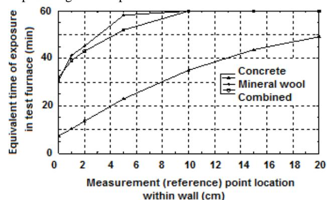
Figure 8 Test furnace equivalent exposure times – 60min room fire
