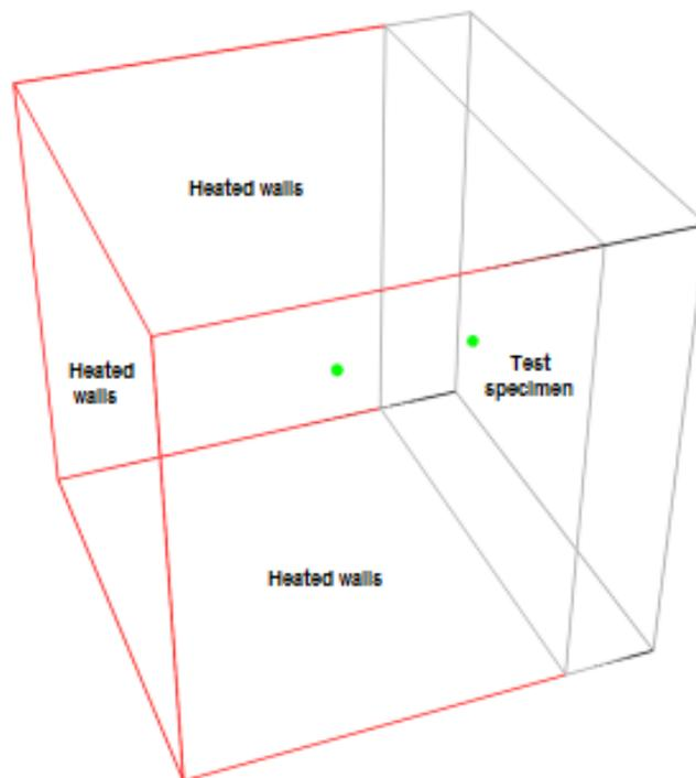
Figure 2 Wireframe visualisation of test furnace model
