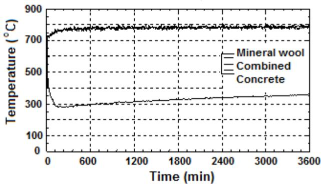
Figure 4 Development of temperatures in room fire simulations
