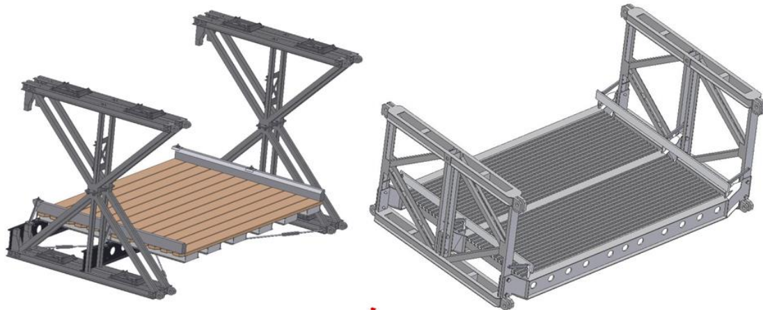
Figure 1: Model of bay TMS and MS bridge set created by Autodesk Inventor SW
