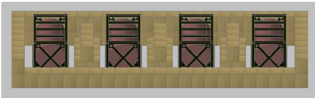
Figure 3: POL store ballistic protection consist of defence walls
