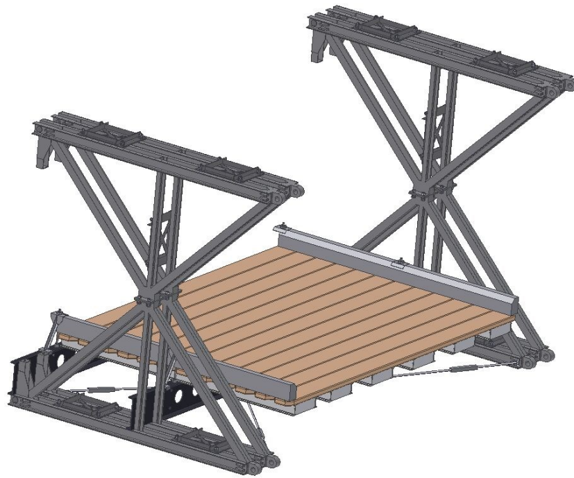
Figure 1. Intermediate bridge bay
